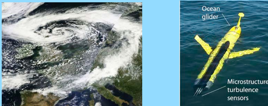
Figure 40: Left: True colour image of Storm Bertha over the North Sea from Aug. 11, 2014, as glider measurements were being made (obtained from NASA World View). Right: Ocean glider on the water surface with microstructure turbulence sensors mounted.
